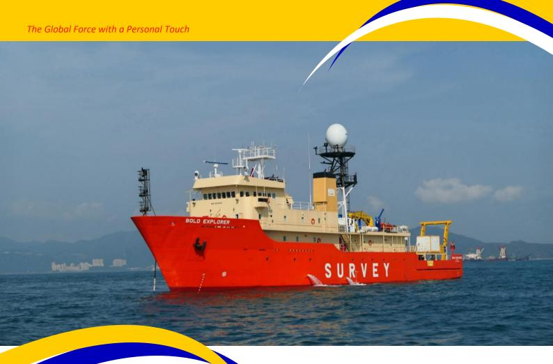
The Bold Explorer is a 68m multi-purpose geophysical and geotechnical survey vessel. This former Stalwart class vessel was fully refitted as a state of the art survey vessel in 2020, by EGS in Singapore.
